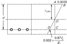
$d = \text{effective depth of beam} \\ x_{u\text{-lim}} = \text{limiting depth of neutral axis} \\ \text{From similar triangles},$
